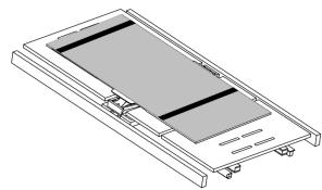
Mount the cover by sliding the pockets over the head end and foot end arms. The head end of the cover contains the label information and placement of the cover symbol:
