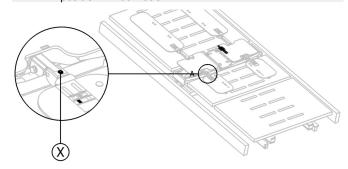
To adjust the position of the arms, fold them up at the joints to the main module and adjust screw  $\circledast$  until the arms are in a horizontal position when folded back down.
