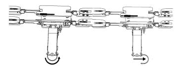
3. After the pin is removed, the motor will fall out of the support, if the motor does not fall out carefully take it out of the support and slowly lower the wing.
