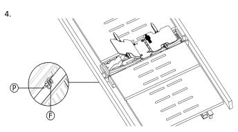
Elevate the wing and secure it and reduce the risk of injuries. Ensure the main modules platform is side aligned with bed support frame. Place the bracket from set  $^{\textcircled{e}}$  in to the designated slots on the main module and fix the main module with the bracket on the bed frame on both sides of the bed. Gradually tighten the bolts  $^{\textcircled{e}}$  with a 4 mm Allen key on both sides.
