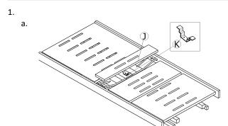
Remove the plastic cover ①, and the metal support ® underneath. On some bed models the metal support ® is fixed with a bolt under the bed some parts from the bed (e.g actuators or covers) need to be removed and placed back, after the metal support is removed.
