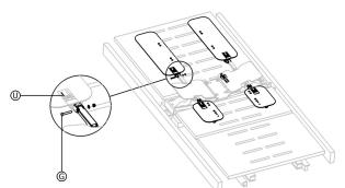
Connect the four arms with the main module, following the representation on the arms label shown in the zoomed image @, the black shaded area on the sticker represents the location were the arm must be placed. Fix the four arms with the Allen bolts from set @ and tighten the lock nuts facing inwards. Ensure the safety washers are placed on the lock nut side.
