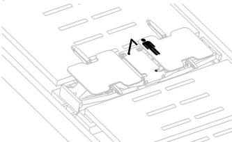
Use a 4 mm Allen key in order to tighten the balance bolts through the holes on top of the middle plate.
