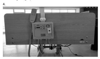
Collect the motor cables in a bundle and tighten it with a zip tie, move the bed up and down to make sure that the bundle is not clinging on any bed parts and moves freely.
