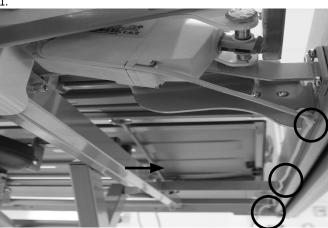
Run the motor cable underneath the bed frame toward the foot end (indicated by the arrow in the image), on both sides of the bed and fix each of the cables with zip ties onto the frame tube. Ensure that both motor cables are tighten with zip ties (marked by the circles in the picture), first zip tie near the motor and the last 2 on the frame tube toward the foot end. Make sure the end of the zip ties, are not facing outwards from the bed frame.
