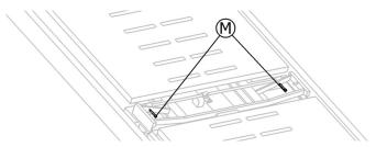
For the Seta Pro bed remove the 2 bolts (M) and reverse them so the head of the bolts face the foot end of the bed, place back and tighten the reversed bolts.
