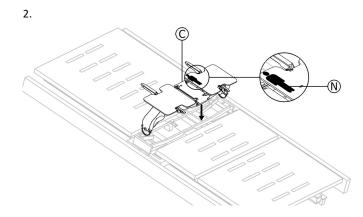
Place the main module C onto the bed, following the symbol represented in the zoomed image R. Head facing towards the head end of the bed and feet towards the foot end of the bed. For certain models the main module does not fit straight down and has to be wiggled onto the bed. Make sure the main module C is pushed all the way towards the head end of the bed.
