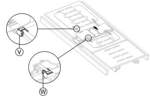
Ensure that the head arms is mounted on the telescopic bracket © in the first threaded hole and you are not able to see the remaining threaded holes. For the foot arms make sure the telescopic bracket ©, is mounted on the third hole and you are able to see 2 threaded holes.
