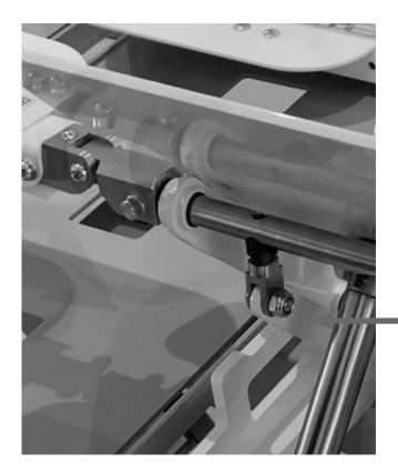
The angle rod assembly can be bended, due to cyclic exposure of high load.
