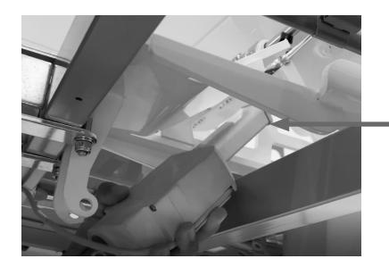
Take out the actuator, if needed losen the actuator cable by cutting the plastic strip that holds it.
