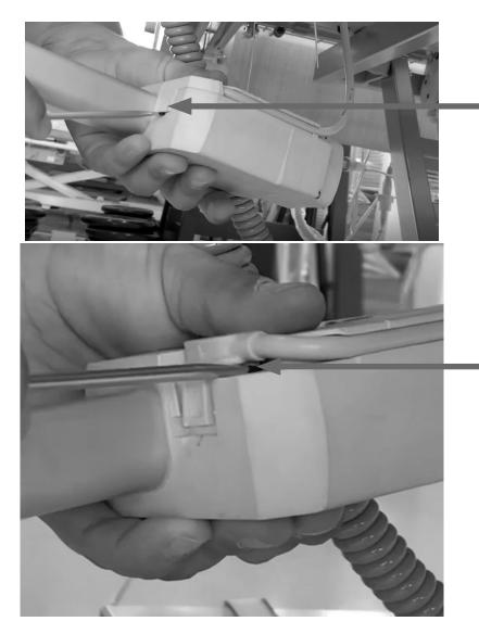
Use the screwdriver to remove the safety plastic from the cable, be careful not to damage the cable.
