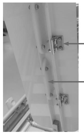
The hinges supporting the top plate on the arms can get damaged. Can be order together with the arm via spare parts.
