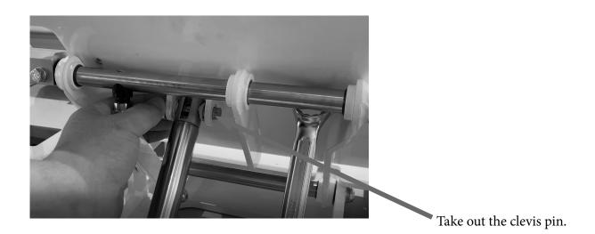
5. Remove the actuator pin
